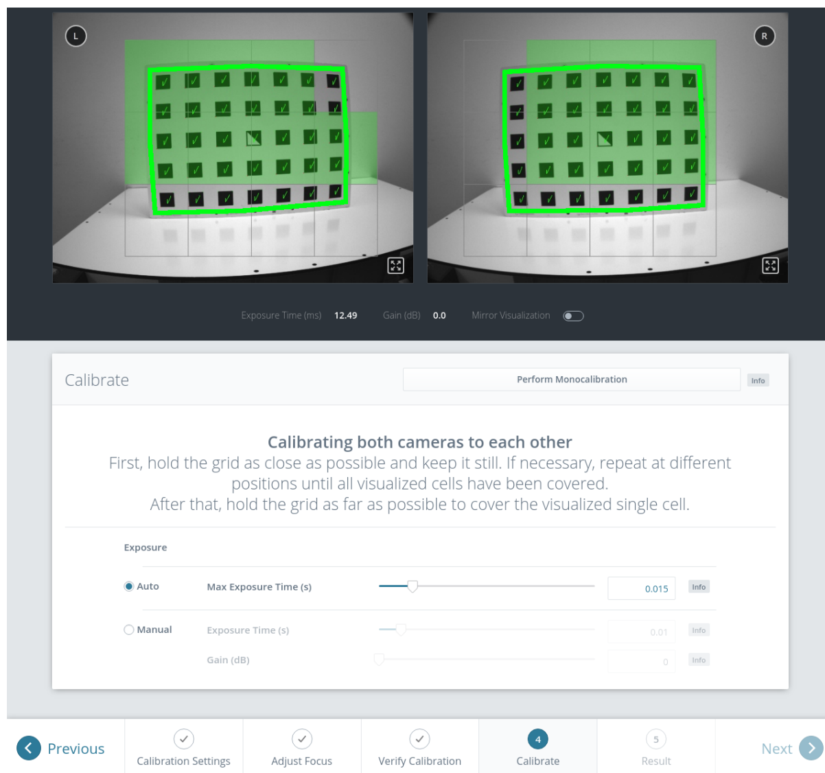
Fig. 5.31: Stereo calibration: Hold the grid as close as possible to fill all visualized cells
